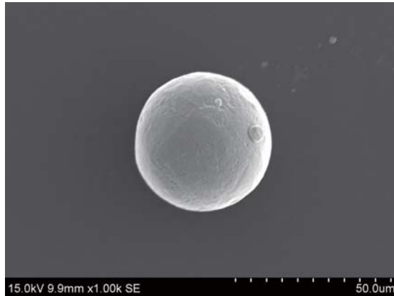
Photo1 - Silicolloy A2 metal powder (1000magnifications)
