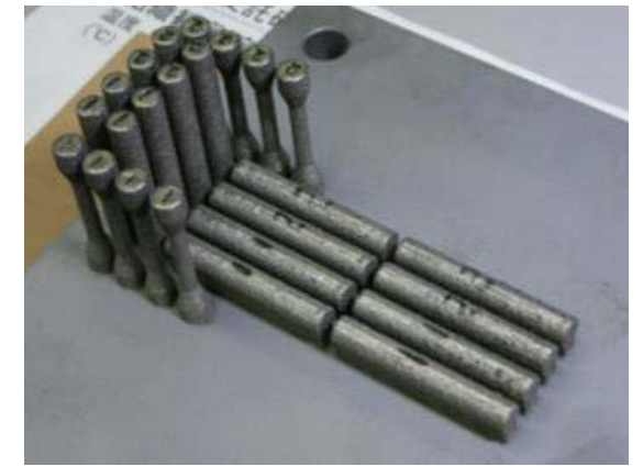
Photo6 - Selective laser sintering Molding to portrait orientation and landscape orientation
